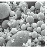
The spherical shape of fly ash improves the concrete qualities by filling the voids between the constituents of the concrete, which reduces the voids & cracks in the concrete.
